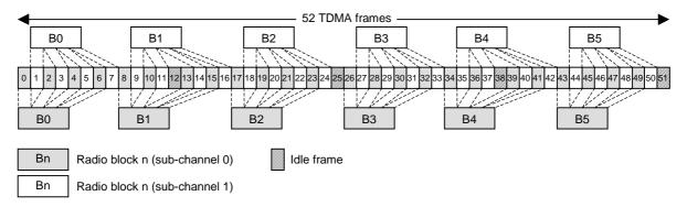
Figure 3: Multiframe structure for PDCH/H
