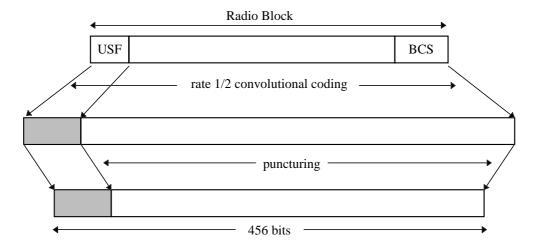
Figure 7: Radio Block structure for CS-1 to CS-3
