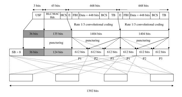
Figure 12: Coding and puncturing for MCS-7; rate 0.76 8PSK, two RLC blocks per 20ms
