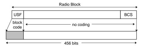
Figure 8: Radio Block structure for CS-4
