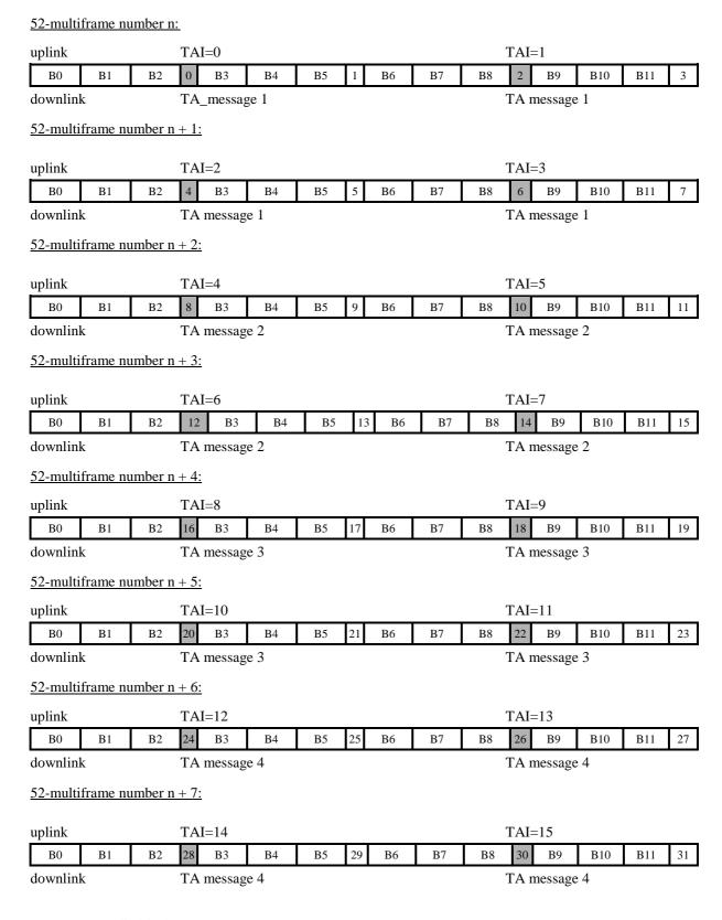
B0 - B11 = Radio blocks Idle frames are numbered from 1 to 31 [odd numbers]
