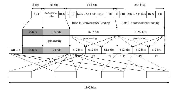
Figure 11: Coding and puncturing for MCS-8; rate 0.92 8PSK, two RLC blocks per 20ms
