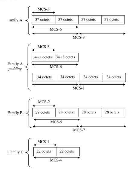
Figure 9: General description of the Modulation and Coding Schemes for EGPRS
