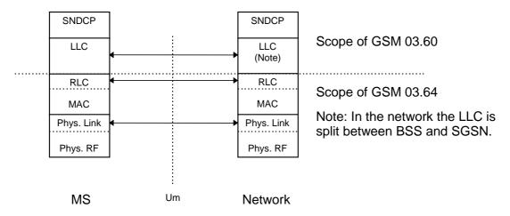
Figure 3d: GPRS MS - Network Reference Model
