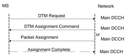
Figure 24b: Access and allocation for the packet request procedure, uplink packet transfer
