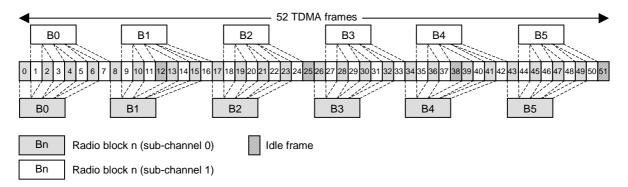
Figure 3: Multiframe structure for PDCH/H
