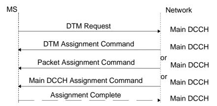
Figure 24b: Access and allocation for the packet request procedure, uplink packet transfer
