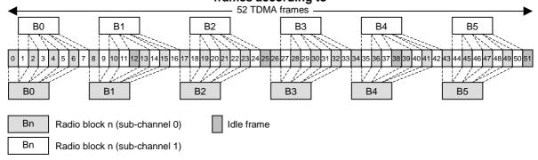
Figure 3. No frames are used for PTCCH (see GSM 05.02 [11]) and the two idle frames can be used by the MS for signal measurements and BSIC identification.
