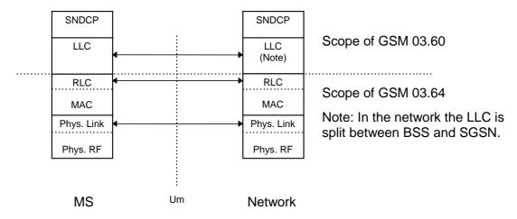
Figure 7: GPRS MS – Network Reference Model
