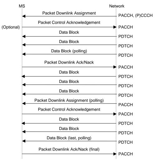
Figure 27: An example of downlink data transfer
