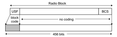
Figure 8: Radio Block structure for CS-4
