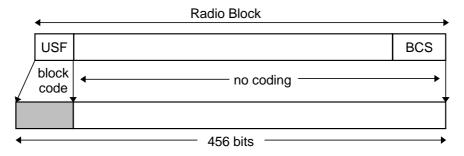
Figure 8: Radio Block structure for CS-4
