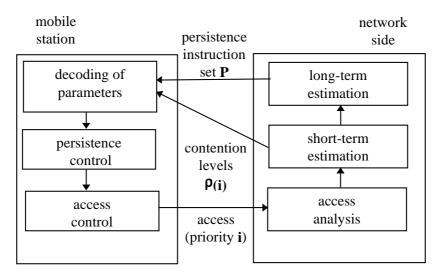
Figure 24: Basic principle of random access traffic control
