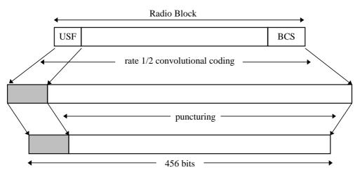
Figure 7: Radio Block structure for CS-1 to CS-3
