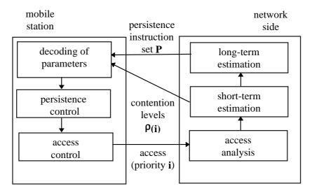
Figure 10: Basic principle of random access traffic control
