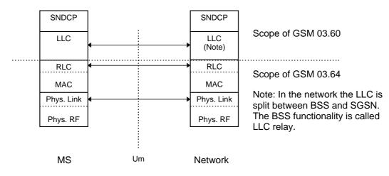
Figure 3: GPRS MS – Network Reference Model
