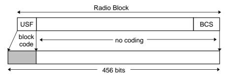
Figure 6: Radio Block structure for CS-4
