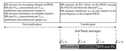
Figure A.2: Traffic example of downlink power control
