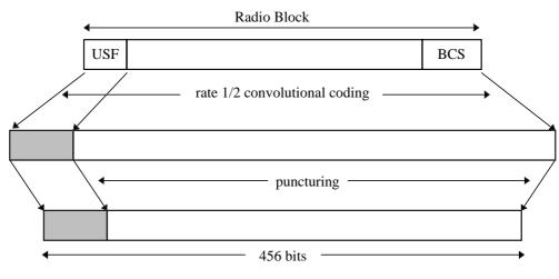
Figure 5: Radio Block structure for CS-1 to CS-3
