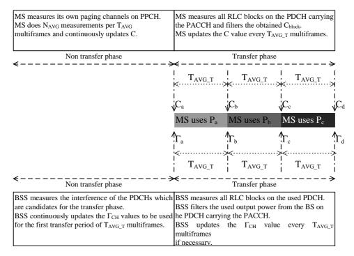
Figure A.1: Traffic example of uplink power control
