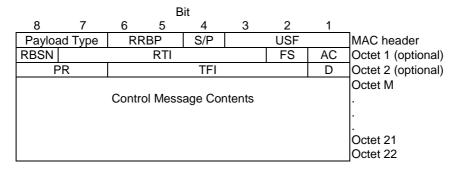
Figure 10.3.1.1: Downlink RLC/MAC control block together with its MAC header
