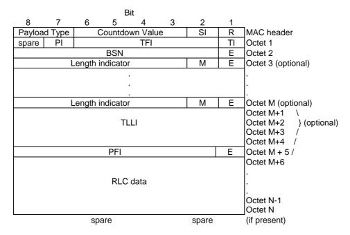
Figure 10.2.2.1: Uplink RLC data block with MAC header
