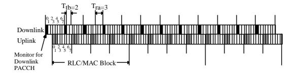
Figure D.3: Multislot Class 3 (Rx=2, Tx=2,Sum=3), 2 timeslot uplink TBF
