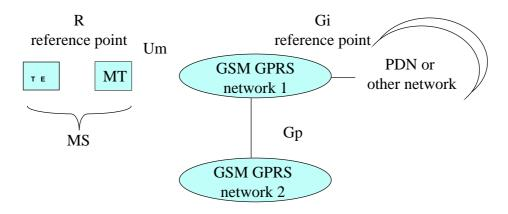
Figure 1: GPRS Access Interfaces and Reference Points
