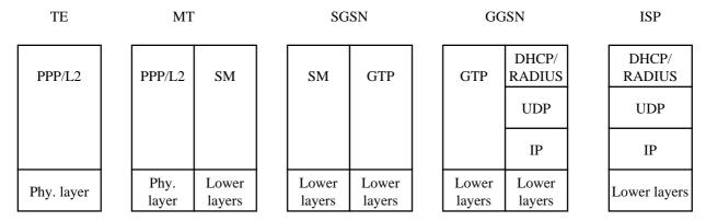
Figure 11: Signalling plane of non transparent case
