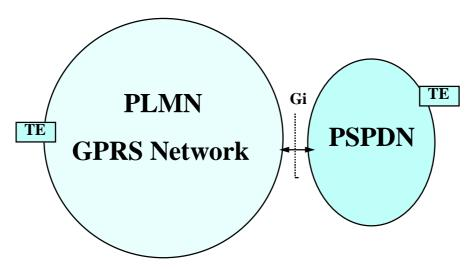
Figure 3: PSPDN Interworking with X.75 at Gi Reference Point
