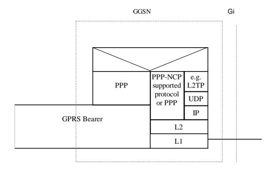
Figure 13: The protocol stacks for the Gi PPP reference point
