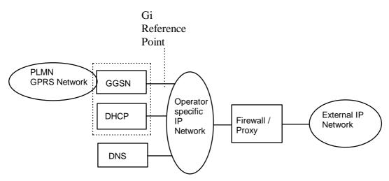
Figure 9: Example of the PDN Interworking Model, transparent case
