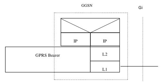
Figure 8: The protocol stacks for the GilP reference point
