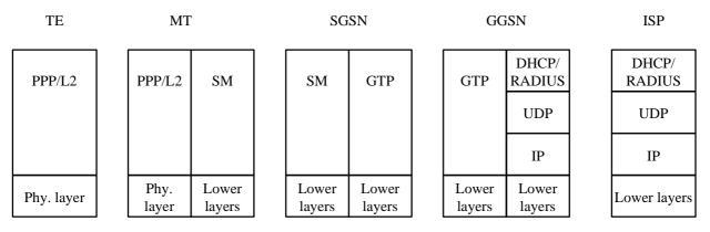
Figure 11: Signalling plane of non transparent case
