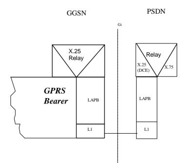
Figure 6: The Protocol Stack for the X.25 / Gi Reference point
