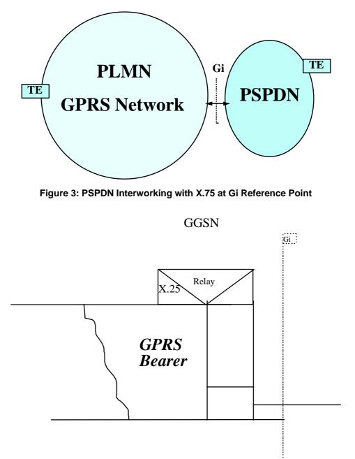
Figure 4: The Protocol Stack for the X.75 Gi Reference Point
