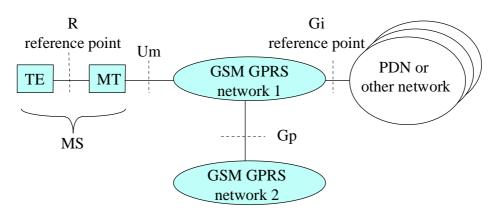
Figure 1: GPRS Access Interfaces and Reference Points
