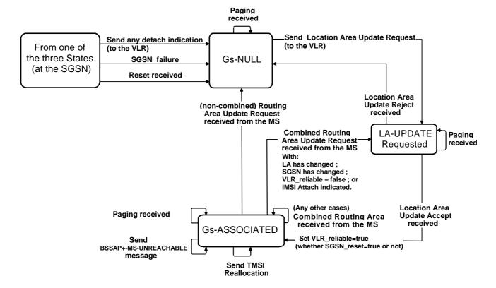
Figure 4.2/GSM 09.18: State diagram at the SGSN
