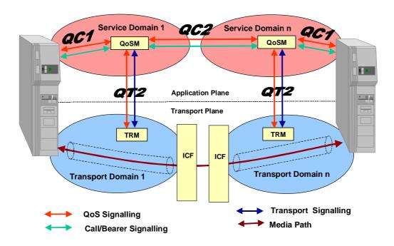
Figure 19: Multiple Service Domains/Multiple Transport Domains - Case II
