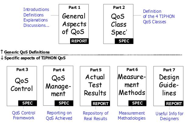
Figure 1: TIPHON WG5 QoS documentation structure
