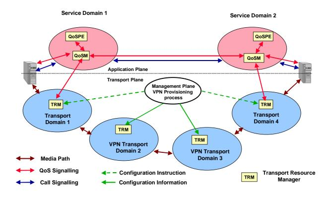
Figure 21: Multiple Service Domains/Multiple Transport Domains - Provisioned VPN
