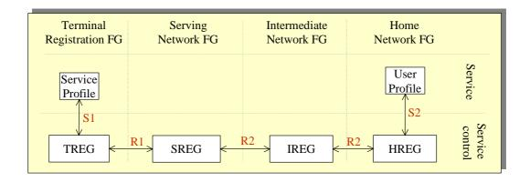
Figure 5.3: Functions involved during the registration of a user
