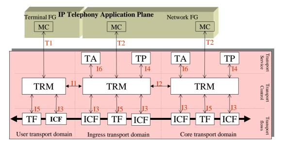
Figure 6.2: Reference points in the IP Transport plane
