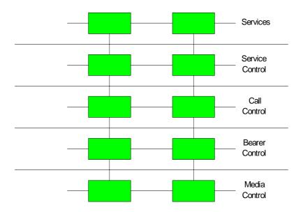
Figure 5.1: Functional layers in the IP Telephony Application plane
