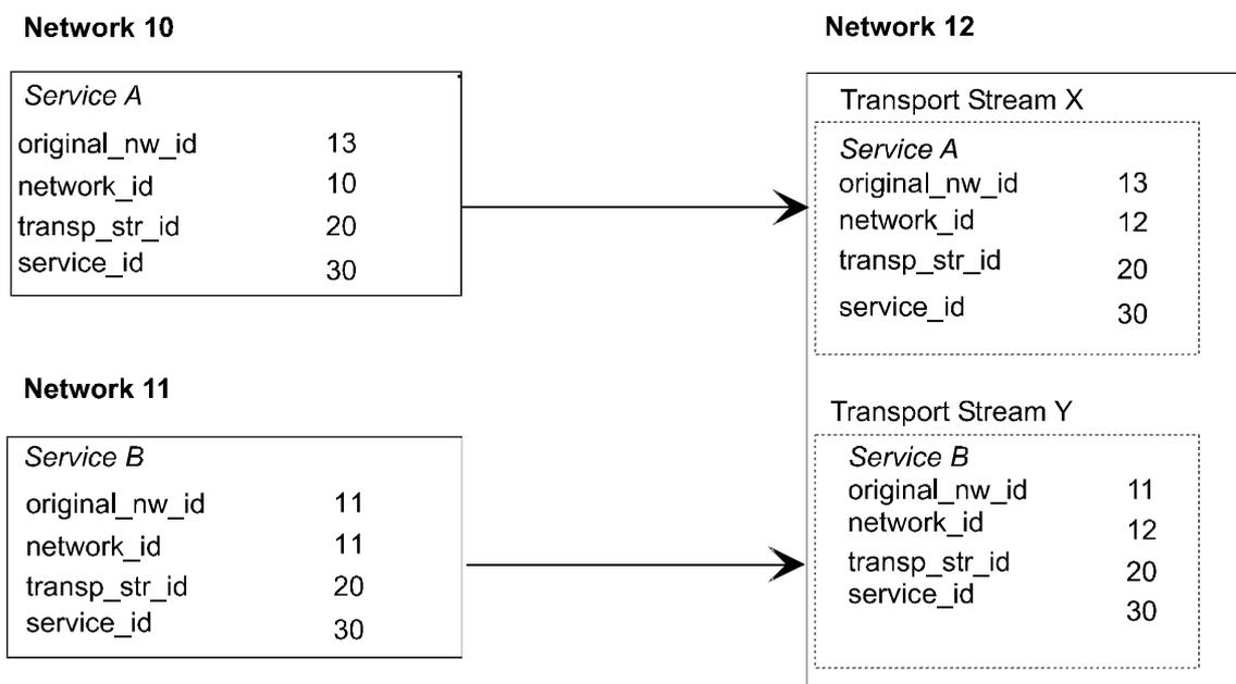
Figure 2: Transfer to a new delivery system
