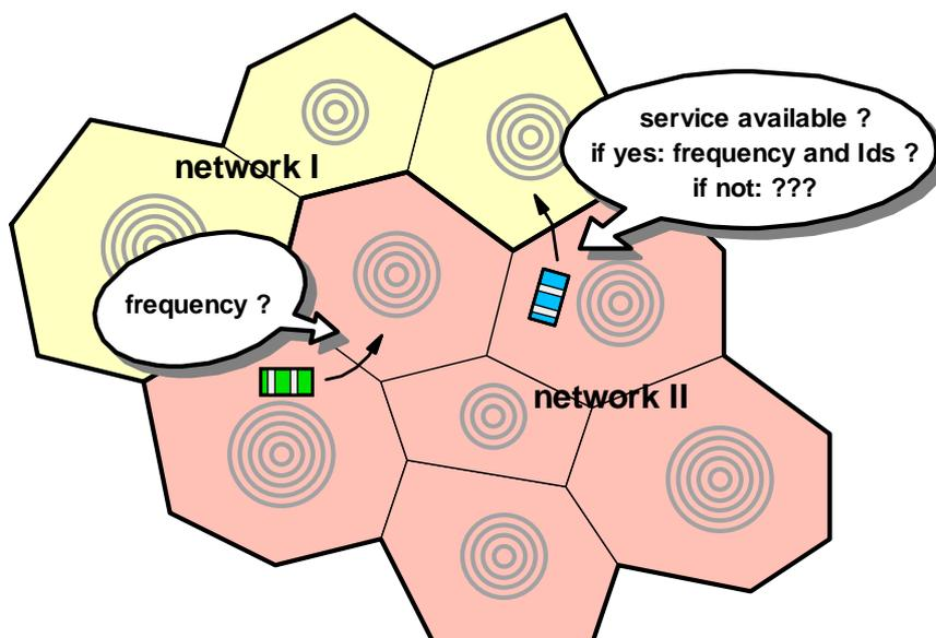
**Figure 6: Hand-over situations in DVB-T networks**
