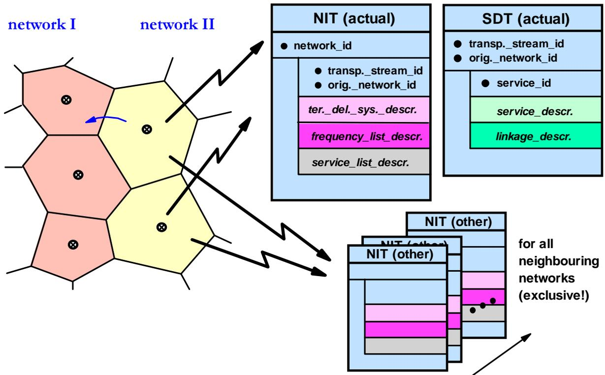
Figure 7: Hand-over at network borders by means of the frequency\_list\_descriptor and the service\_list\_descriptor
