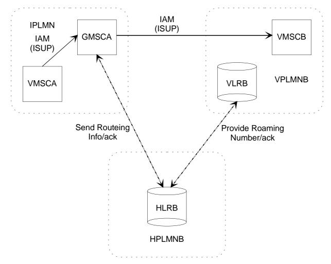
Figure 1: Architecture for optimal routeing of basic mobile-to-mobile call
