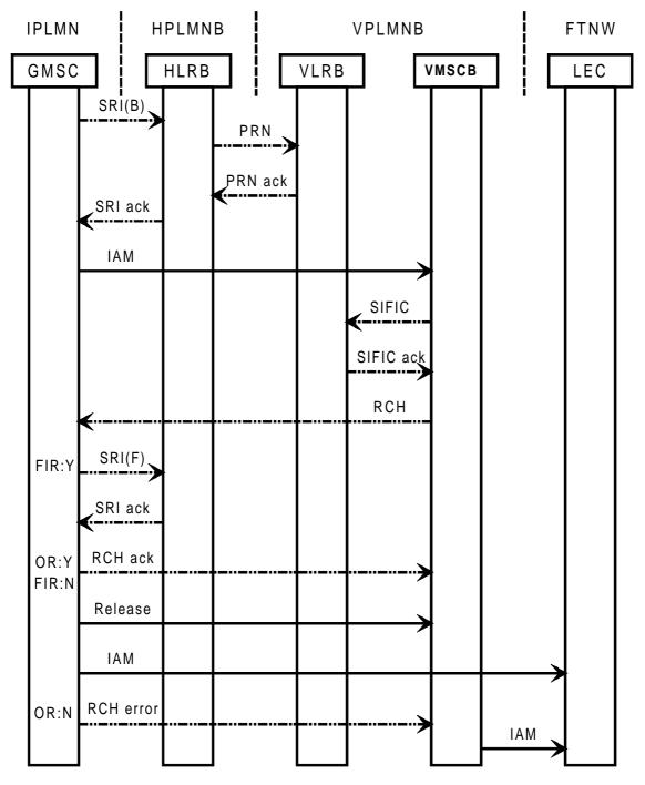
Figure 5: Message flow for optimal routeing of late call forwarding to a fixed destination
