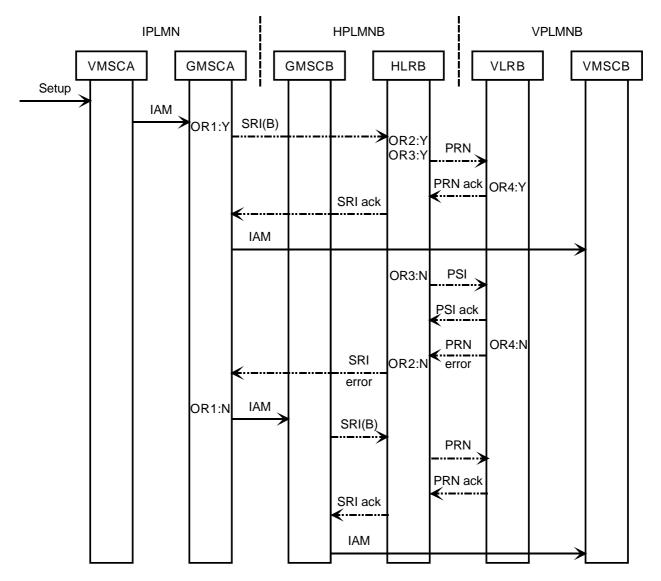
Figure 3: Message flow for optimal routeing of basic mobile-to-mobile call
