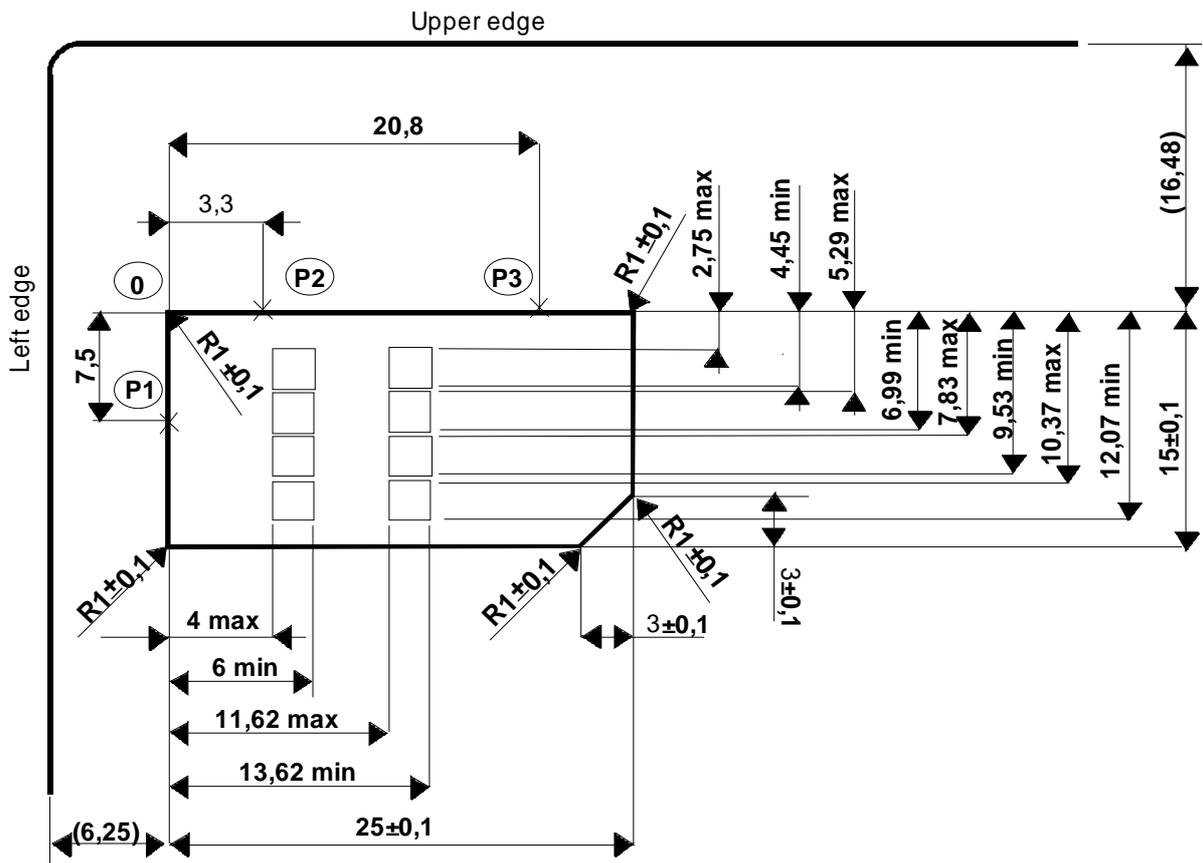
NOTE: The Plug-in SIM may be "obtained" by cutting away excessive plastic of an ID-1 SIM. The values in parenthesis in figure A.1 show the positional relationship between the Plug-in and the ID-1 SIM and are for information only.
