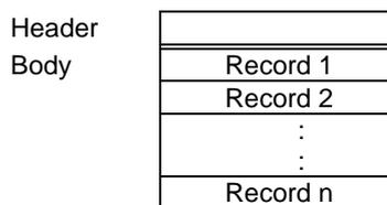
**Figure 5: Structure of a linear fixed file**
