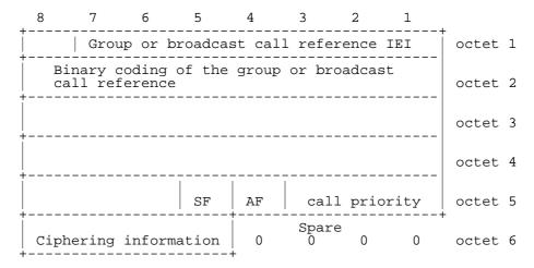
Figure 10.5.8/GSM 04.08: Descriptive Group or Broadcast Call Reference
