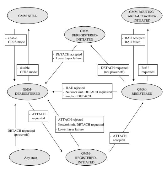
Figure 4.1b/GSM 04.08: GMM main states in the MS
