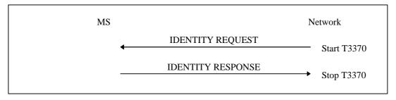
Figure 4.7.8/1 GSM 04.08: Identification procedure
