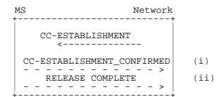
Figure 5.7a/GSM 04.08: Call initiation and possible subsequent responses
