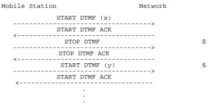
Figure 5.9/GSM 04.08: Multiple DTMF transmission
