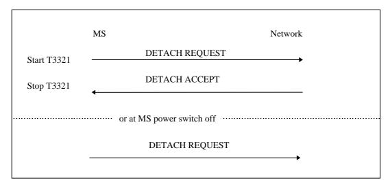
Figure 4.7.4/1 GSM 04.08: MS initiated GPRS detach procedure
