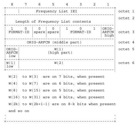
Figure 10.5.38/GSM 04.08: Frequency List information element (Range 256 format)
