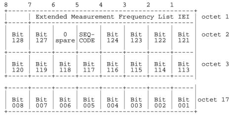
Figure 10.5.74/GSM 04.08: Extended Measurement Frequency List information element
