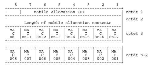
Figure 10.5.49/GSM 04.08: Mobile Allocation information element
