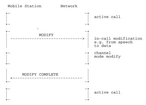
Figure 7.17/GSM 04.08: In-call modification
