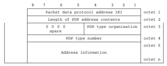
Figure 10.5.137/GSM 04.08: Packet data protocol address information element
