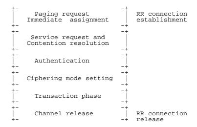
Figure 7.1/GSM 04.08: Components of structured procedures
