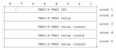
Figure 10.5.70/GSM 04.08: TMSI/P-TMSI information element
