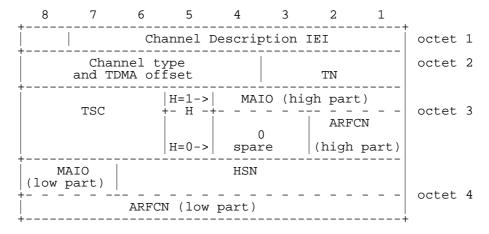
Figure 10.5.25/GSM 04.08: Channel Description information element
