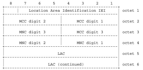
Figure 10.5.3/GSM 04.08: Location Area Identification information element
