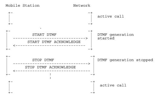
Figure 7.13/GSM 04.08: DTMF protocol control
