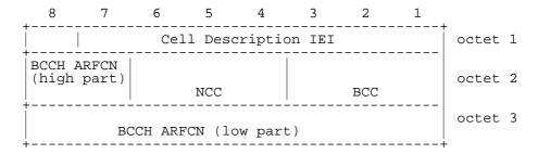
Figure 10.5.20/GSM 04.08: Cell Description information element
