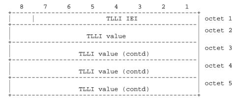
Figure 10.5.69/GSM 04.08: TLLI information element
