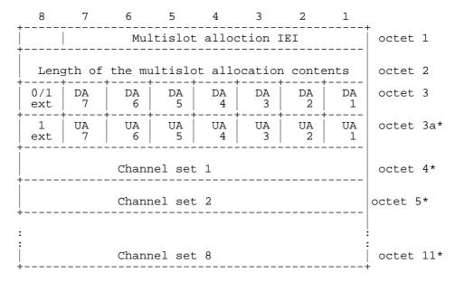
Figure 10.5.51/GSM 04.08: Multislot Allocation information element
