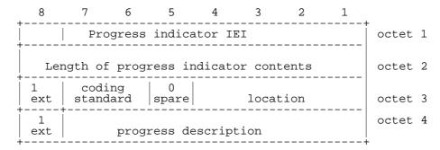
Figure 10.5.107/GSM 04.08: Progress indicator information element
