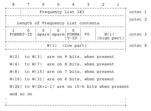
Figure 10.5.36/GSM 04.08: Frequency List information element (Range 1024 format)
