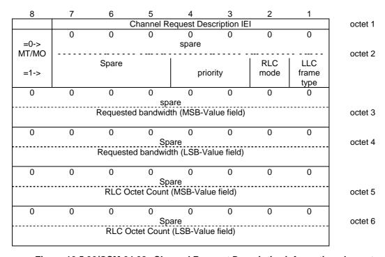
Figure 10.5.30/GSM 04.08: Channel Request Description information element
