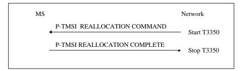
Figure 4.7.6/1 GSM 04.08: P-TMSI reallocation procedure
