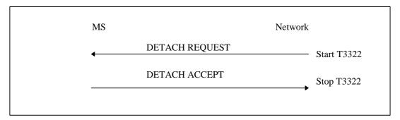
Figure 4.7.4/2 GSM 04.08: Network initiated GPRS detach procedure
