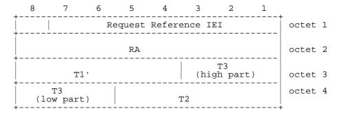
Figure 10.5.61/GSM 04.08: Request Reference information element
