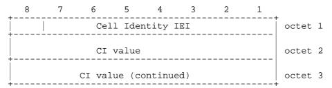
Figure 10.5.1/GSM 04.08: Cell Identity information element
