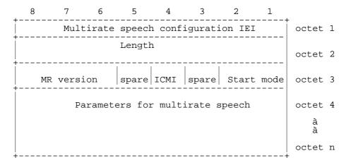
Figure 10.5.2.47/GSM 04.08: MultiRate configuration information element
