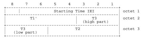
Figure 10.5.65/GSM 04.08: Starting Time information element
