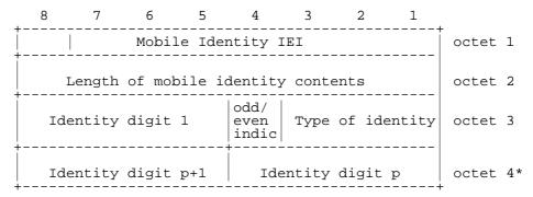
Figure 10.5.4/GSM 04.08: Mobile Identity information element
