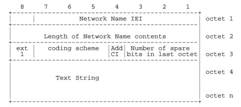
Figure 10.5.80/GSM 04.08: Network Name information element
