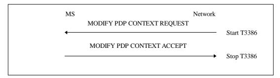
Figure 6.5/GSM 04.08: PDP context modification procedure
