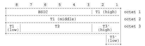
Figure 9.3/GSM 04.08: Frame synchronization information element
