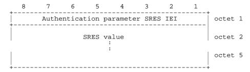
Figure 10.5.76/GSM 04.08: Authentication Parameter SRES information element
