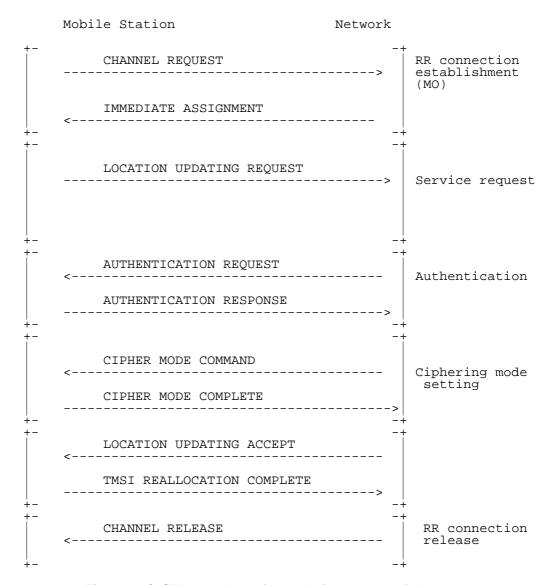
Figure 7.9/GSM 04.08: Location updating: successful case
