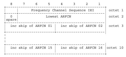
Figure 10.5.34/GSM 04.08: Frequency Channel Sequence information element
