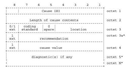
Figure 10.5.95/GSM 04.08: Cause information element
