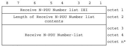
Figure 10.5.127/GSM 04.08: Receive N-PDU Number list information element
