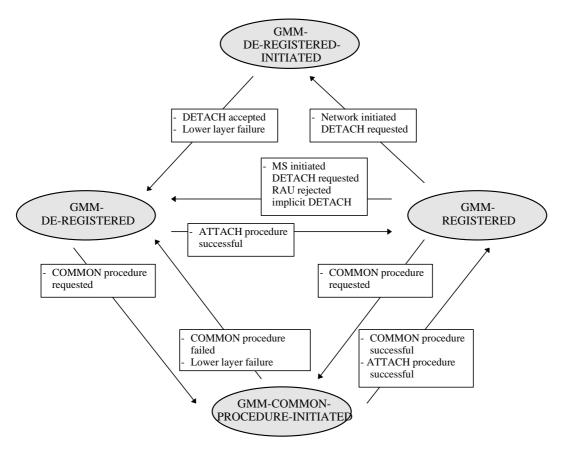
Figure 4.1c/GSM 04.08: GMM main states on the network side
