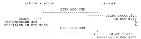
Figure 3.3/GSM 04.08: Ciphering mode setting sequence
