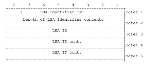
Figure 10.68c/GSM 04.08: LSA Identifier information element
