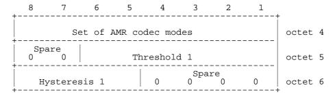
Figure 10.5.2.47b/GSM 04.08: Parameters for multirate speech field for the MR version 1 when a set with two codec modes is chosen
