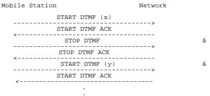
Figure 5.9/GSM 04.08: Multiple DTMF transmission
