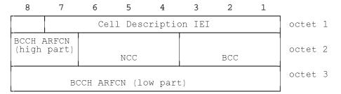
Figure 10.16/GSM 04.08: Cell Description information element
