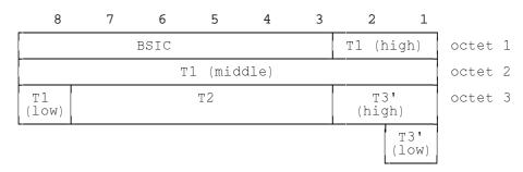
Figure 9.3/GSM 04.08: Frame synchronization information element
