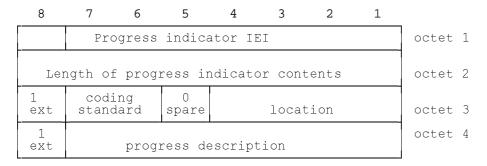
Figure 10.88/GSM 04.08: Progress indicator information element
