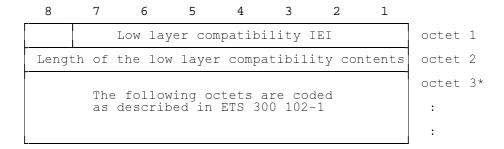
Figure 10.85/GSM 04.08: Low layer compatibility information element
