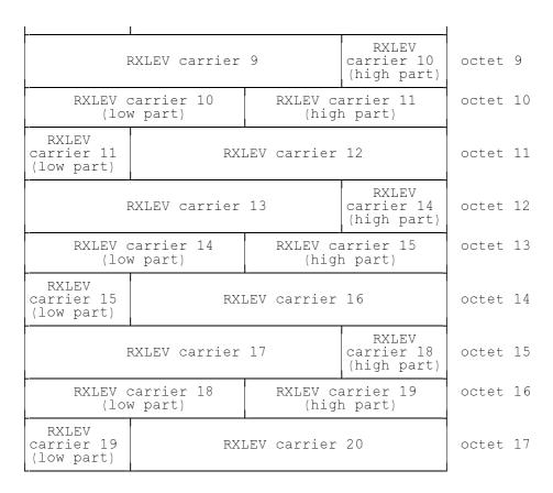
Figure 10.5.2.45.1/GSM 04.08: Extended Measurement Results information element
