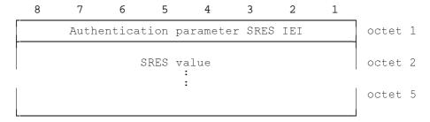
Figure 10.62/GSM 04.08: Authentication Parameter SRES information element
