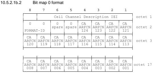
Figure 10.10/GSM 04.08: Cell Channel Description information element, bit map 0 format
