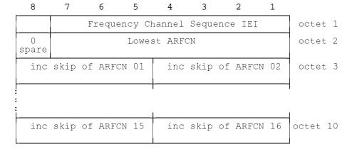
Figure 10.26/GSM 04.08: Frequency Channel Sequence information element
