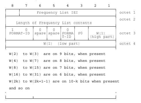
Figure 10.28/GSM 04.08: Frequency List information element (Range 1024 format)
