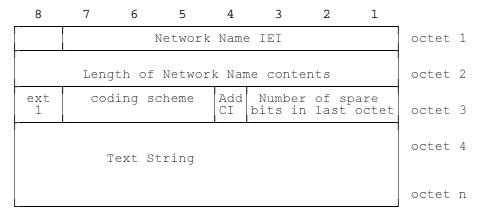
Figure 10.65a/GSM 04.08: Network Name information element
