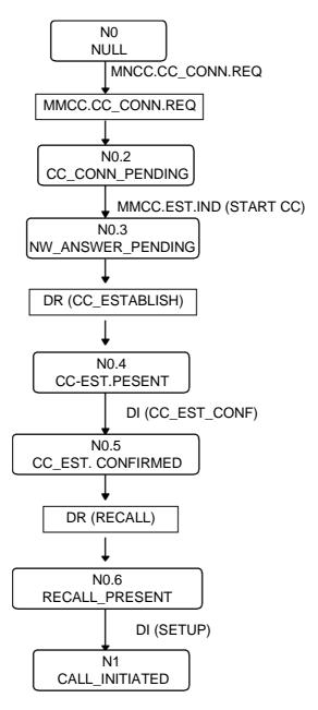
FIGURE 5.1b.1/GSM 04.08: Overview call control protocol/Network side, extension
