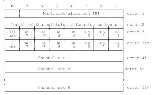
Figure 10.39b /GSM 04.08: Multislot Allocation information element
