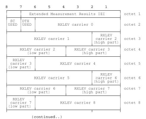
Figure 10.5.2.45.1/GSM 04.08: Extended Measurement Results information element
