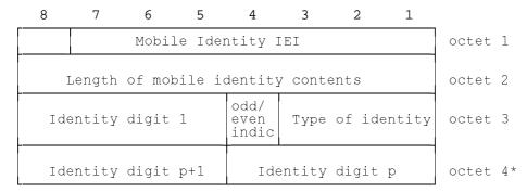
Figure 10.5/GSM 04.08: Mobile Identity information element
