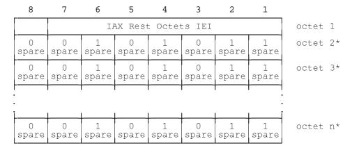
Figure 10.36/GSM 04.08: IAX Rest Octets information element
