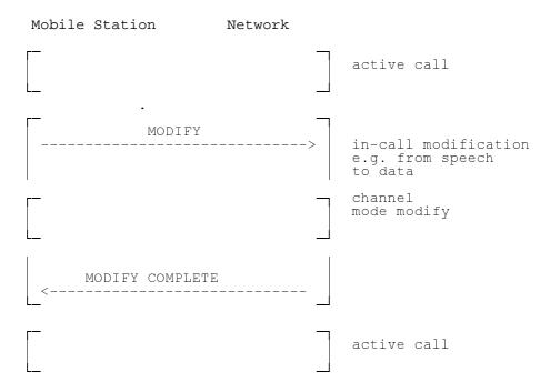
Figure 7.17/GSM 04.08: In-call modification
