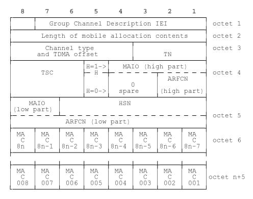
Figure 10.32a/GSM 04.08: Group Channel Description information element
