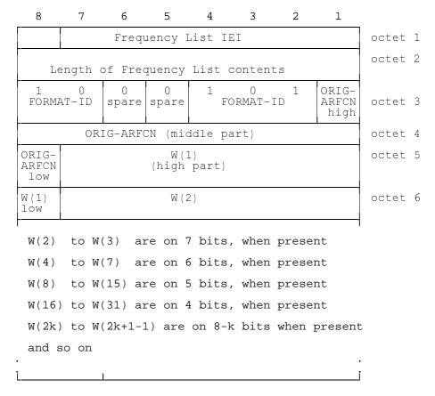
Figure 10.30/GSM 04.08: Frequency List information element (Range 256 format)
