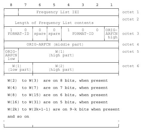
Figure 10.29/GSM 04.08: Frequency List information element (Range 512 format)
