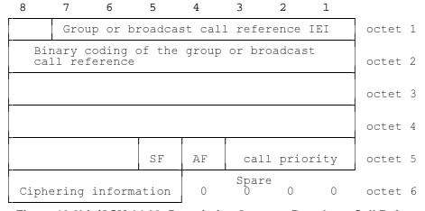
Figure 10.8bis/GSM 04.08: Descriptive Group or Broadcast Call Reference
