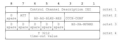
Figure 10.25/GSM 04.08: Control Channel Description information element
