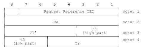
Figure 10.48/GSM 04.08: Request Reference information element
