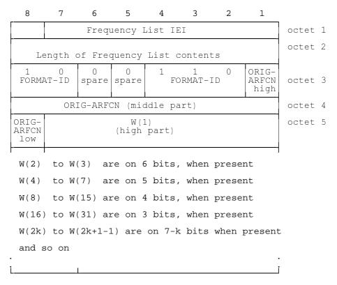
Figure 10.31/GSM 04.08: Frequency List information element (Range 128 format)
