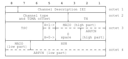
Figure 10.19/GSM 04.08: Channel Description information element
