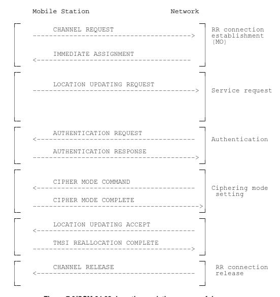
Figure 7.9/GSM 04.08: Location updating: successful case
