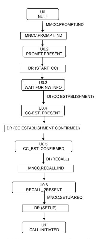
Figure 5.1a.1/GSM 04.08: Overview call control protocol/MS side, extension
