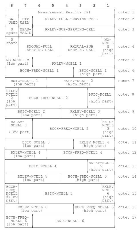
Figure 10.38/GSM 04.08: Measurement Results information element (continued)
