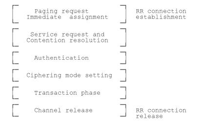
Figure 7.1/GSM 04.08: Components of structured procedures
