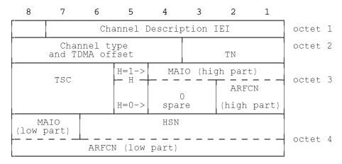
Figure 10.19a/GSM 04.08: Channel Description 2 information element
