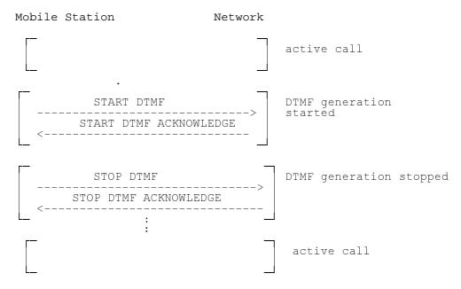
Figure 7.13/GSM 04.08: DTMF protocol control
