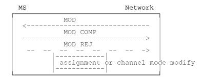
Figure 5.10b/GSM 04.08: In-call modification sequence initiated by network
