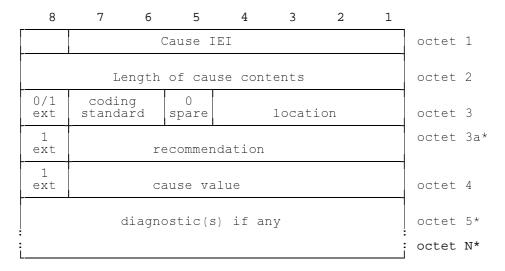
Figure 10.77/GSM 04.08: Cause information element
