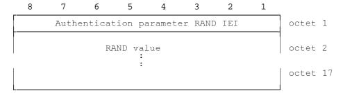
Figure 10.61/GSM 04.08: Authentication Parameter RAND information element
