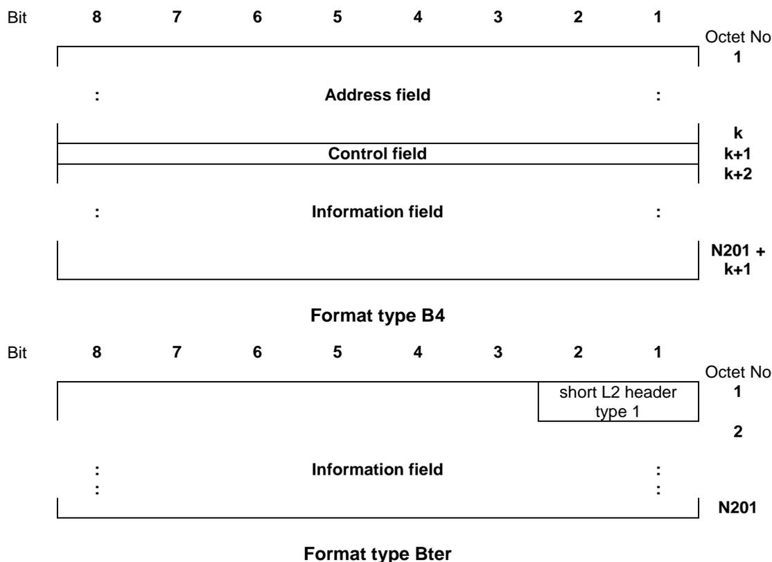
Figure 1/3GPP TS 04.06 (sheet 3 of 3): General frame formats
