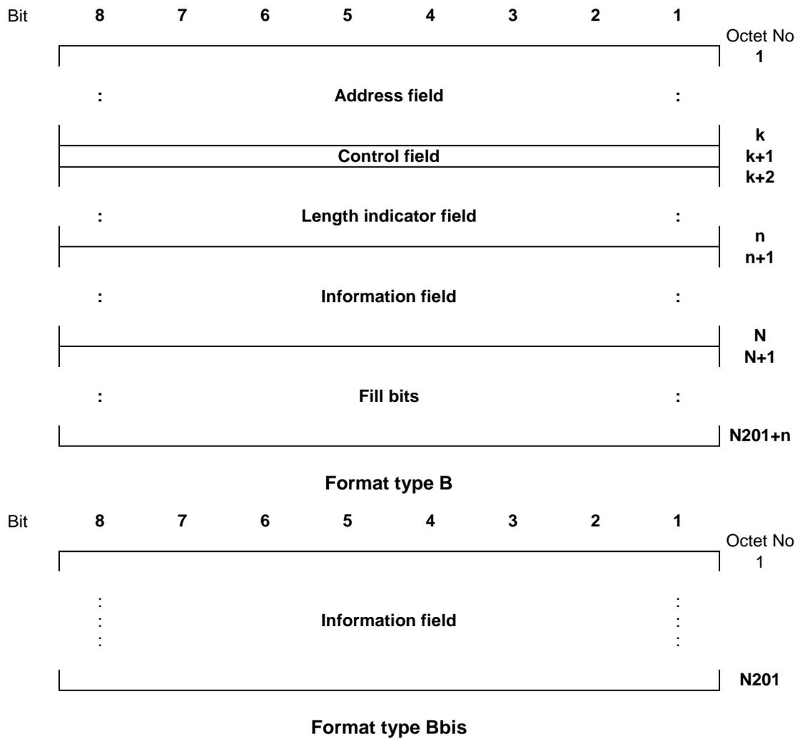
Figure 1/3GPP TS 04.06 (sheet 2 of 3): General frame formats
