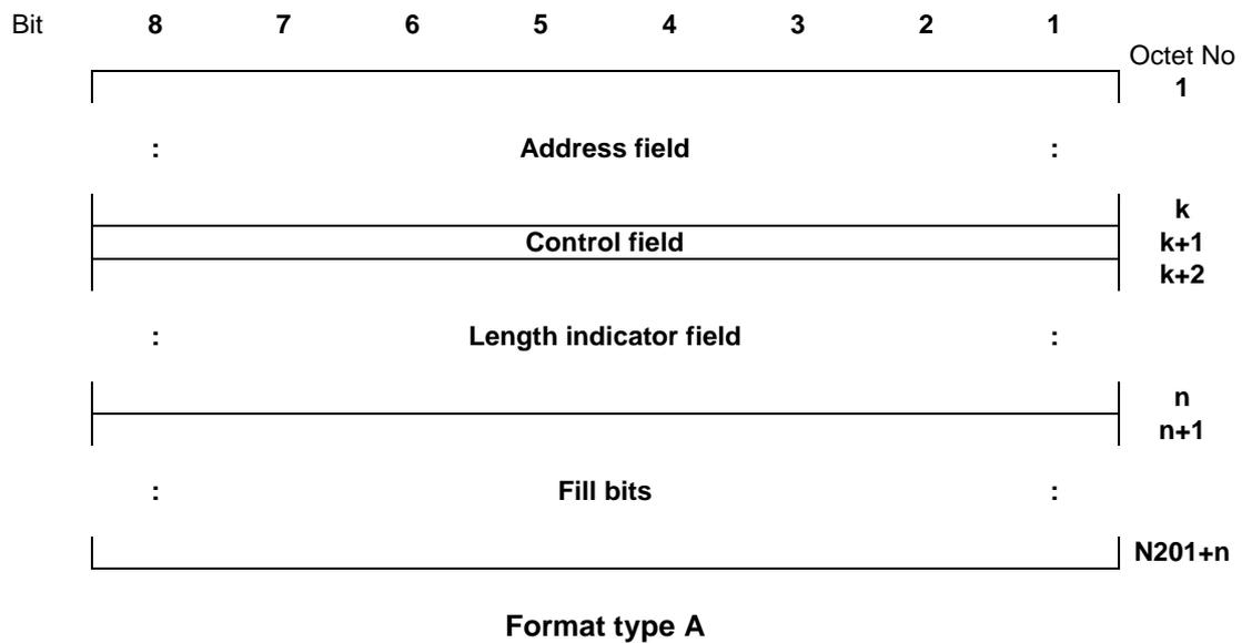
**Figure 1/3GPP TS 04.06 (sheet 1 of 3): General frame formats**
