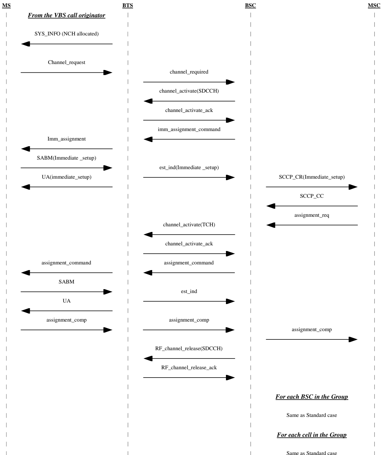
Figure 4a: Signalling information required for establishing voice broadcast calls by a service subscriber using immediate setup
