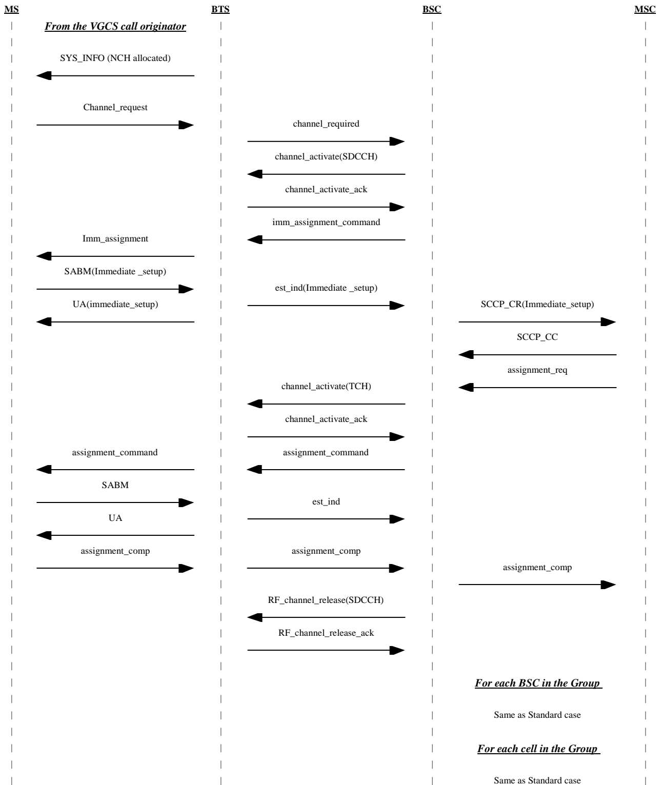
Figure 7a: Signalling information required for establishing voice group calls by a service subscriber using immediate setup
