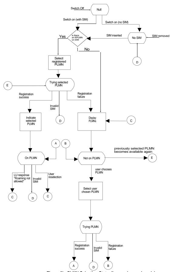
Figure 2b: PLMN Selection State diagram (manual mode)
