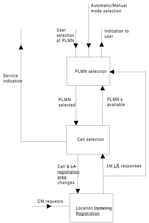
Figure 1: Overall Idle Mode process
