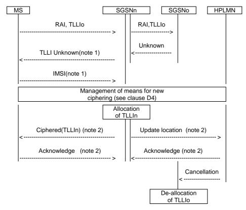
NOTE 1: From a security point of view, the exact signalling messages (described in GSM 03.60) used to indicate that the TLLI is unknown, or to send the IMSI are irrelevant.
