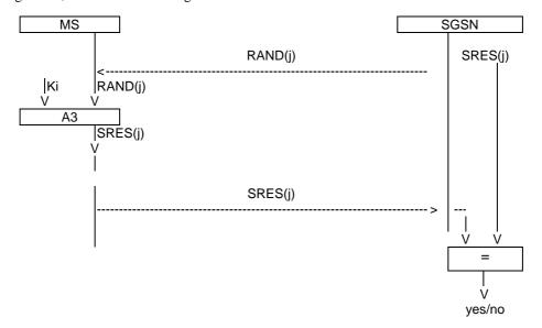
Figure D.3.3: General authentication procedure
