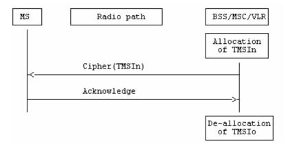
Figure 2.5: Reallocation of a new TMSI
