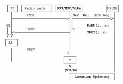
Figure 3.5: Authentication at location updating in a new VLR, using IMSI
