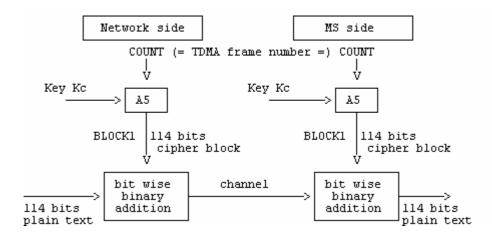
Figure C.2: Deciphering on the MS side
