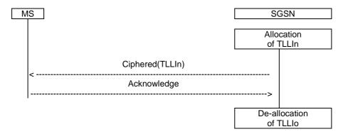
Figure D.2.4: Reallocation of a new TLLI
