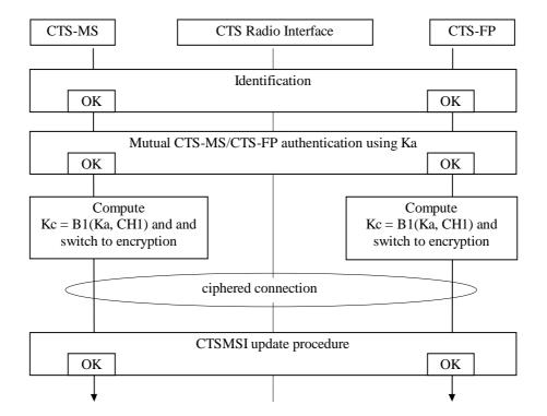
Figure E5: The general access procedure
