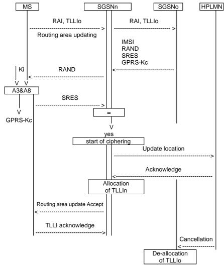
Figure D.5.1: Routing area updating procedure
