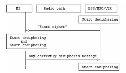
Figure 4.2: Starting of the enciphering and deciphering processes
