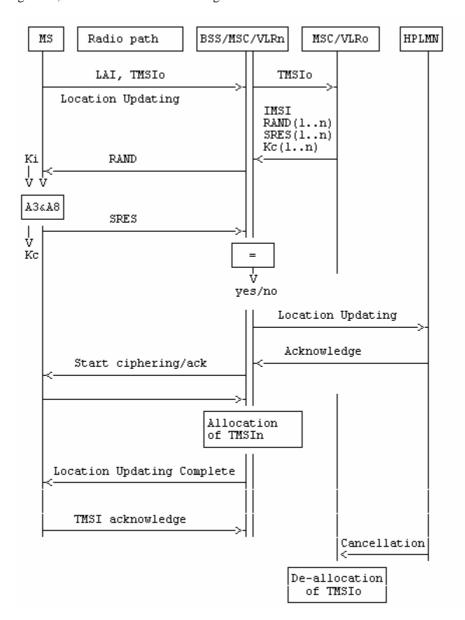
Figure 5.1: Normal location updating procedure
