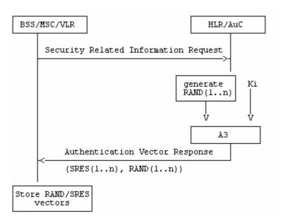
Figure 3.2: Procedure for updating the vectors RAND/SRES
