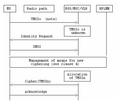
NOTE: Any message in which TMSIo is used as an identifying means in a location area managed by the same VLR.
