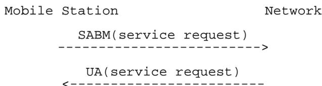
**Figure 7.4/GSM 04.08 Service request and contention resolution**
