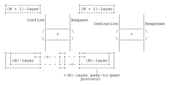
Figure 5: Primitive action sequence for peer-to-peer communication
