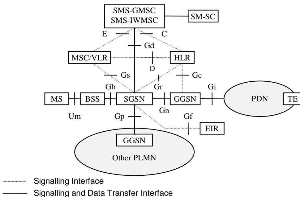
**Figure 2: Configuration of a PLMN supporting GPRS**
