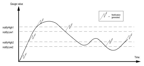
Figure 4: Example gauge threshold behaviour
