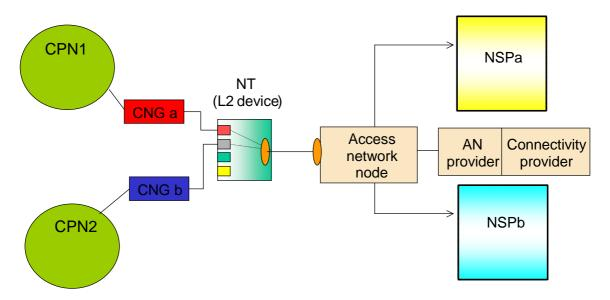
Figure 4: Customer network architecture for multiple gateways, multiple service providers
