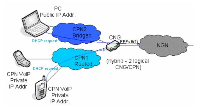
Figure 2: Hybrid model with separate physical networks
