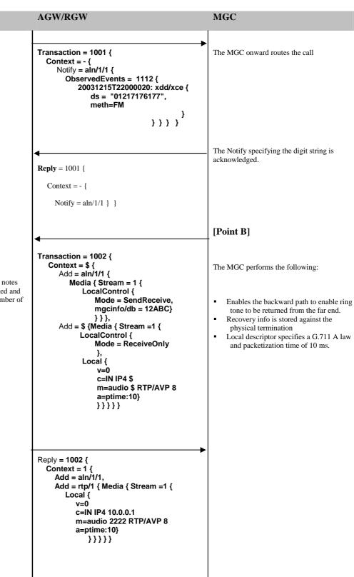
The AGW/RGW creates a context and notes that receive only path has been requested and fills in the IP address and RTP port number of the local descriptor.
