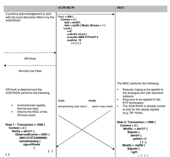
Since the "Off-Hook" has crossed over with the "Ring", the MGC determines that a Call Collision has occurred and the outgoing call has priority. The AGW will be unable to apply Alerting or Ringing Tone because Party A is Off-Hook and will report an error.
