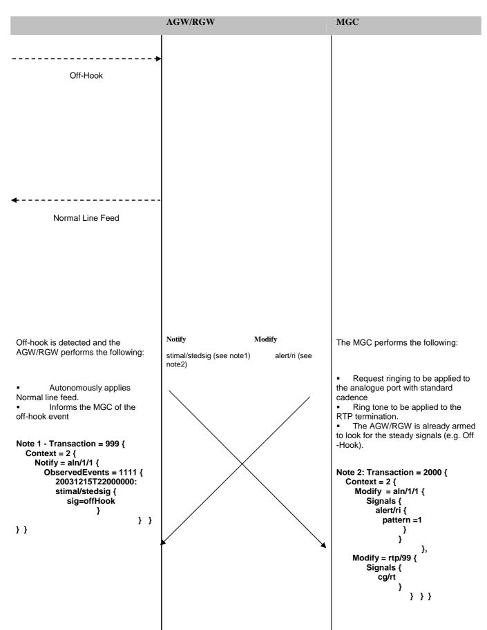
Since the "Off-Hook" has crossed over with the "Ring", then the MGC determines that a Call Collision has occurred and the outgoing call has priority.
