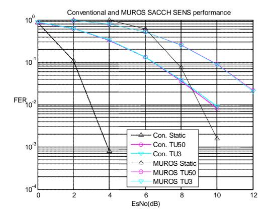
Figure 6-25: DARP Phase 1 mobile SACCH sensitivity performance with static, TU3, TU50 channels and iFH on non-MUROS and MUROS (C1/AWGN)
