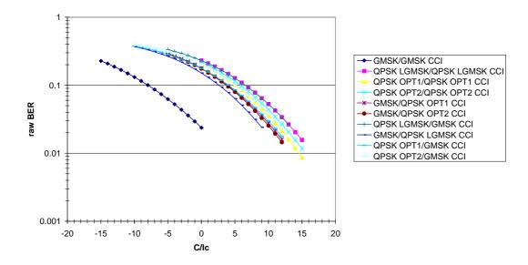
Figure 7-38f. C/I performance for different types of co-channel interference in a VAMOS I receiver.
