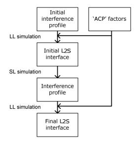
Figure 7-38e. L2S modelling methodology used in the investigation.
