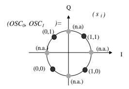
Figure 7-1: Mapping of OSC modulating bits into 8PSK symbols.
