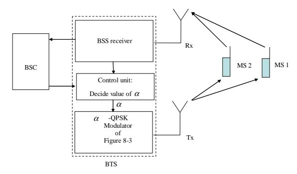
Figure 8-4: Adaptive  $\alpha$  -QPSK modulator
