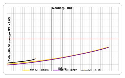
Figure 7-38c. Bad Quality Call for the Non-DARP receiver for MUROS-2 50%.
