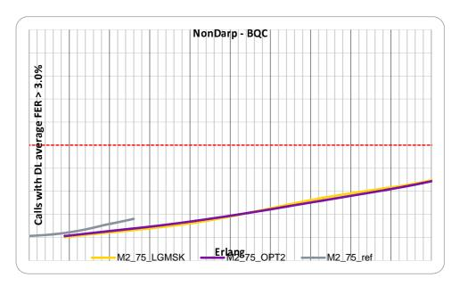
Figure 7-38d. Bad Quality Call for the Non-DARP receiver for MUROS-2 75%.
