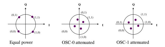
Figure 7-4: Illustration of OSC signals after SAIC processing by MS in neighbour cell
