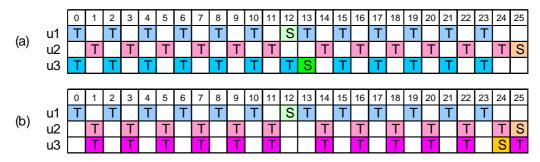
Figure 11-4: Shifted SACCH with three half rate TCHs
