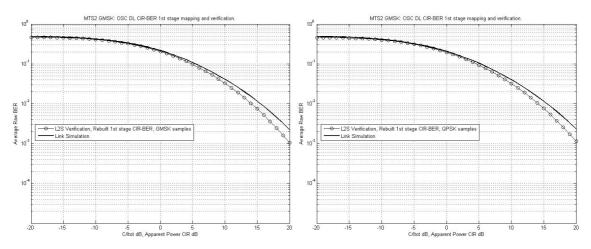
Figure 39-z. Mapping verification using GMSK interferers (left) and QPSK interferers (right).
