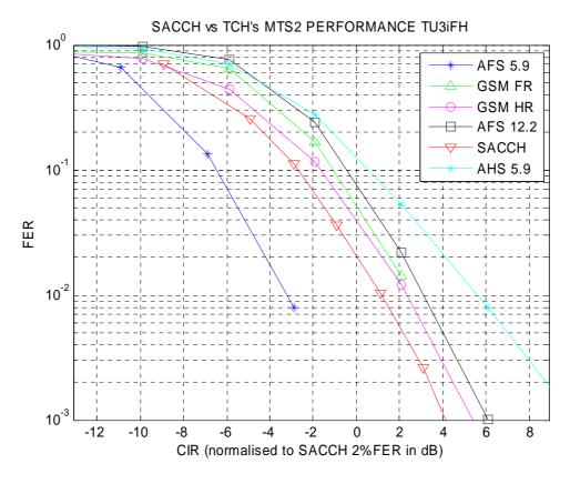
Figure 6-30: DARP Phase 1 mobile SACCH/TCH's performance in MTS-2 scenario with TU3 iFH
