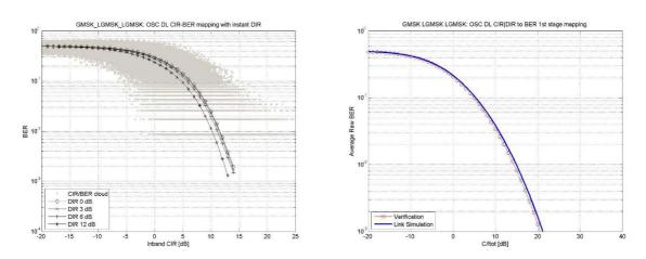
Figure 39-e. Mapping and verification for a GMSK modulated carrier
