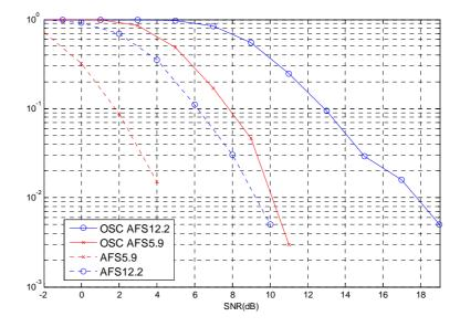
Figure 7-9: DL sensitivity FER performance in HT100iFH of generic DARP phase 1 MS receiving an OSC sub channel with AMR FR 5.9 and 12.2
