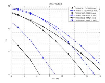
Figure 7-31: DL Asynchronous Co-channel interference performance (MTS3) of a legacy DARP MS receiving a MUROS sub channel using AMR half rate 5.9, AMR full rate 12.2 and AMR full rate 5.9
