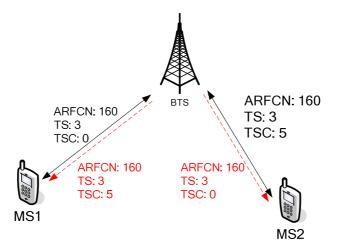
Figure 6-1 Channel assignment for co-TCH operation
