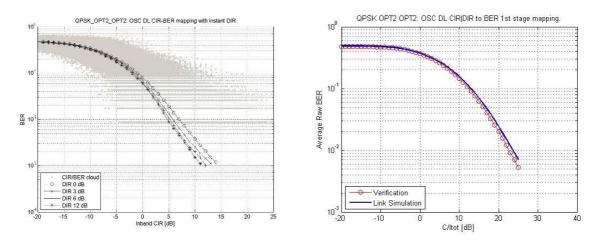
Figure 39-x. Mapping and verification for a QPSK modulated carrier
