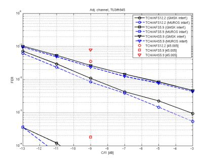
Figure 7-35: Adjacent channel interference performance (lower band) of a legacy DARP MS receiving a MUROS sub channel using AMR half rate 5.9, AMR full rate 12.2 and AMR full rate 5.9
