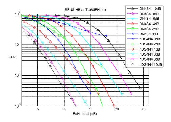
Figure 6-24: MUROS mode performance of DARP mobile with power imbalance in AWGN (GSM HR)
