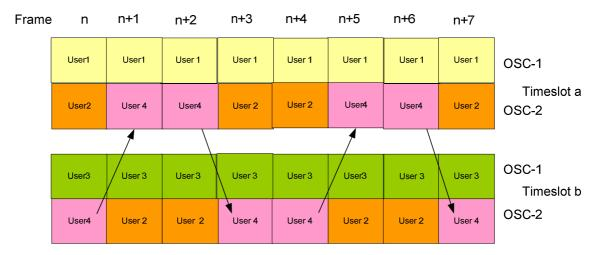
Figure 7-5: Optimized User Diversity for OSC full rate channel configuration for the case of a timeslot pair
