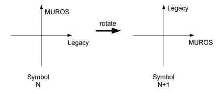
Figure 9-3: π/2 constellation rotation for legacy multiplexing
