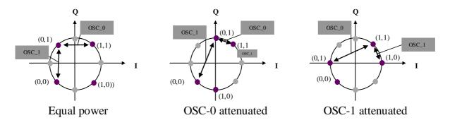
Figure 7-3: Mapping of OSC sub channels with equal or unequal sub channel powers
