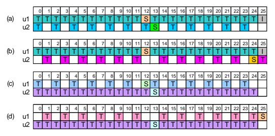
Figure 11-2: Shifted SACCH with one full rate TCH and one half rate TCH
