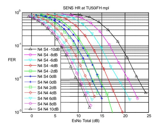
Figure 6-20: MUROS mode performance of DARP mobile with power imbalance in AWGN (GSM HR)
