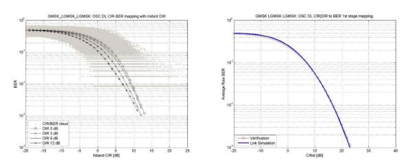
Figure 39-q. Mapping and verification for a GMSK modulated carrier
