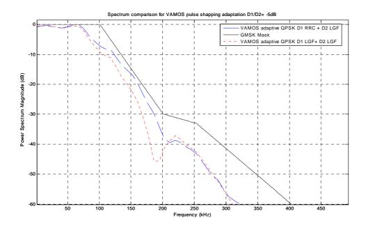
Figure 6-7c - VAMOS spectrum satisfies the GMSK mask: Spectrum of adaptive QPSK VAMOS signal with a RRC pulse shaping on weak signal and a linearised Gaussian pulse shaping (LGF) on strong signal – power imbalance 5dB.
