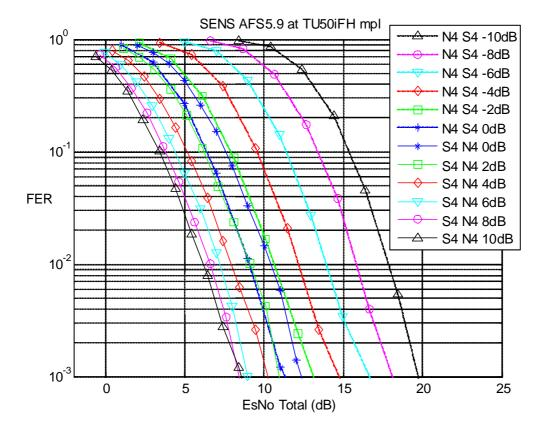
Figure 6-19: MUROS mode performance of DARP mobile with power imbalance in AWGN (AFS 5.9)
