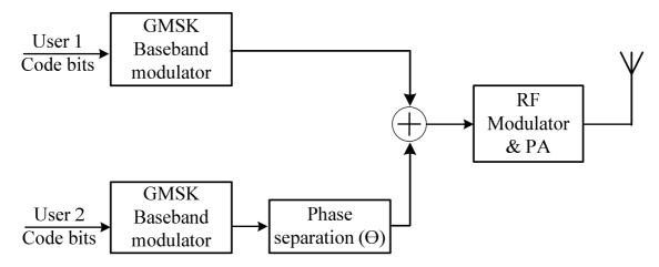
Figure 6-2 Linear baseband combining for co-TCH
