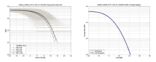
Figure 39-c. Mapping and verification for a GMSK modulated carrier
