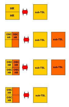
Figure 7-40: Mapping of HR and OSC HR radio channels onto 16 kbit/s Abis sub timeslots
