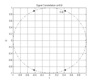
Figure 8-1: Example  $\,lpha$  -QPSK constellation
