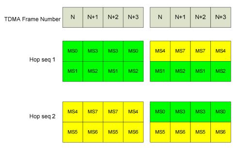
Figure 9-13: Hopping across 2 hopping sequences on Uplink
