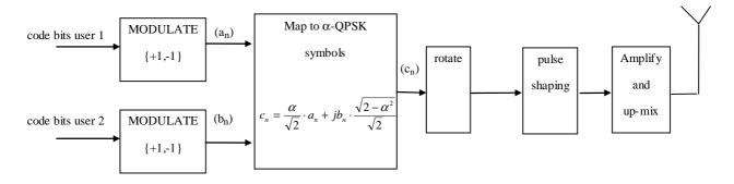
Figure 8-3:  $\alpha$  -QPSK modulator and transmitter
