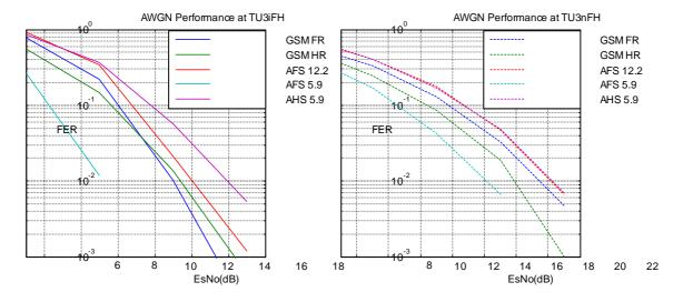
Figure 6-9: DARP Phase 1 mobile performance in sensitivity condition with TU3
