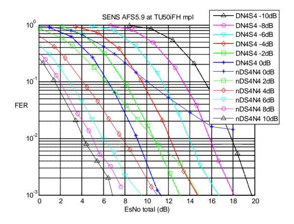
Figure 6-23: MUROS mode performance of DARP mobile with power imbalance in AWGN (AFS5.9)
