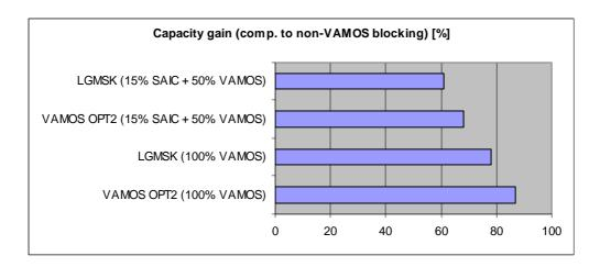
Figure 7-38d2. Capacity gains for MUROS-2 (taken from [7-26]).
