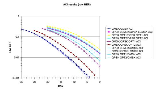
Figure 7-38g. C/I performance for different types of adjacent channel interference in a VAMOS I receiver.
