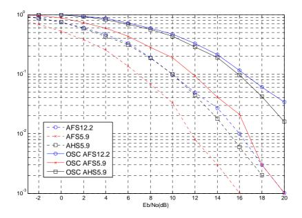
Figure 7-6: DL sensitivity FER performance in TU3nFH of generic DARP phase 1 MS receiving an OSC sub channel with AMR FR 5.9, 12.2 and AMR HR 5.9
