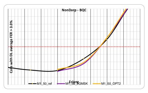
Figure 7-38a. Bad Quality Call for the Non-DARP receiver for MUROS-1 50%.
