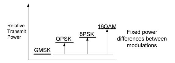
Figure 9-7: Pre-defined Backoff for DTX modulation changes
