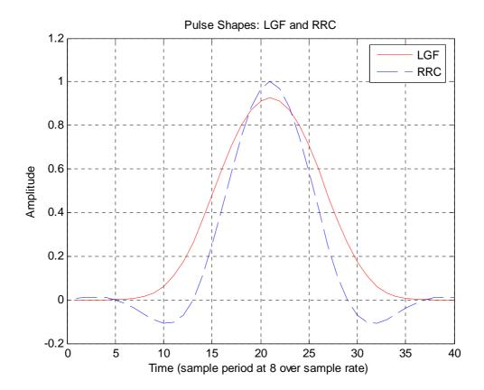
Figure 6-7b - Two pulse shaping used in VAMOS adaptation
