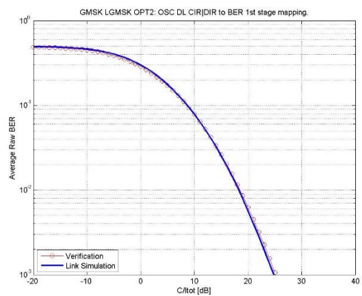
Figure 39-w. Mapping and verification for a GMSK modulated carrier
