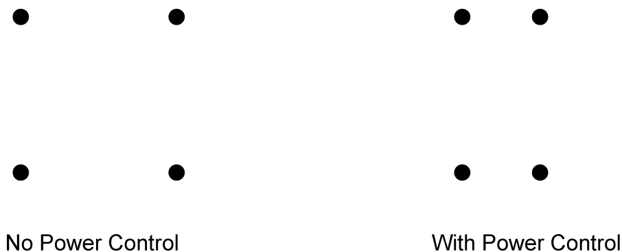
Figure 9-5: Downlink power control on HOM – QPSK
