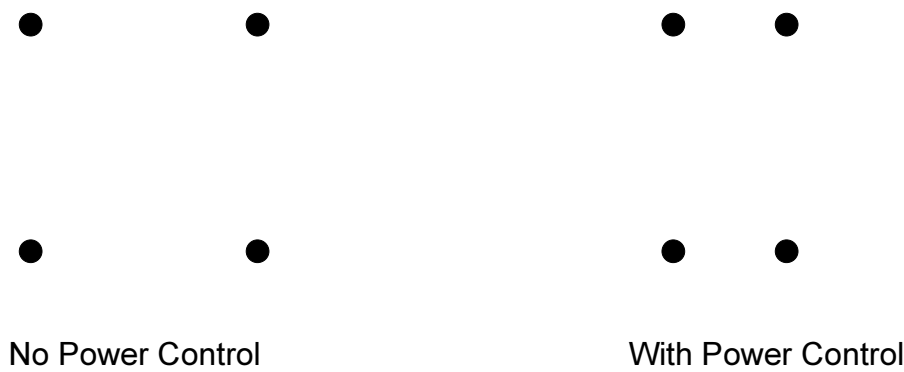
Figure 9-5: Downlink power control on HOM – QPSK
