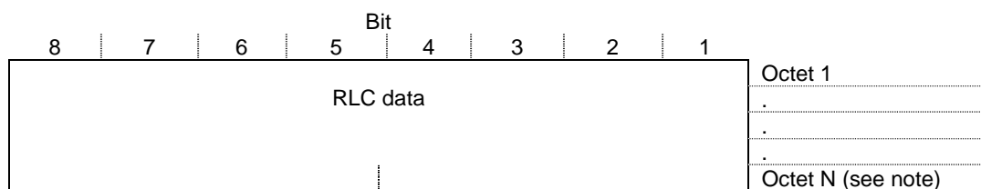
Figure 14: Uplink RLC/MAC block for data transfer in RLC transparent mode
