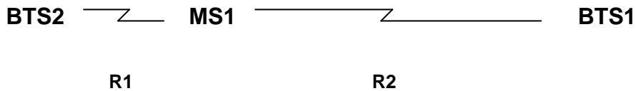
Figure X.9: Representation of relative geometry for BTS intra/inter modulation performance
