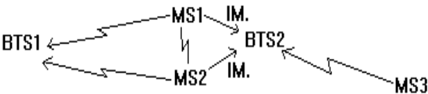
Out-of-band intermods; MS1 and MS2 at full power. Received signal at MS3 from BTS2 at reference sensitivity. By symmetry, MS1 will be affected by an I.M. product from MS2 and MS3 whenever MS3 is affected as shown above.
