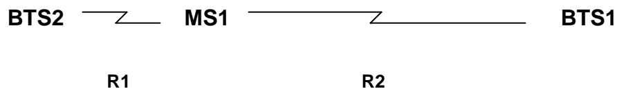
Figure U.2.1: Intra BTS intermodulation performance analysis
