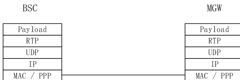
Figure 6.1.1.2.1: User Plane: AoIP protocol stack
