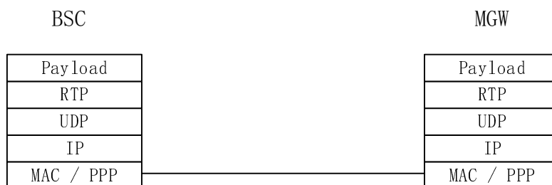
Figure 6.1.1.2.1: User Plane: AoIP protocol stack
