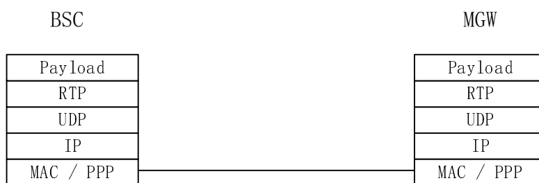
Figure 6.1.1.2.1: User Plane: AoIP protocol stack
