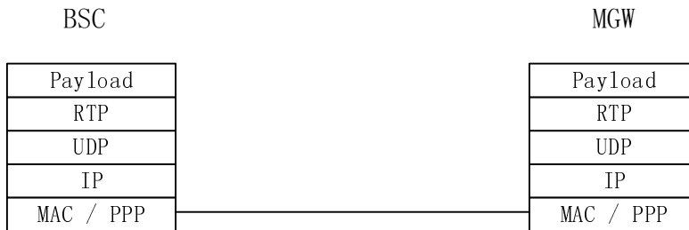
Figure 6.1.1.2.1: User Plane: AoIP protocol stack
