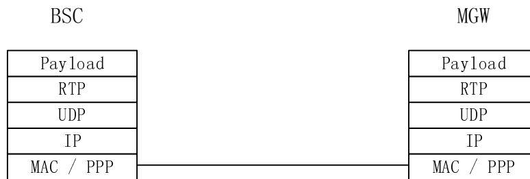
Figure 6.1.1.2.1: User Plane: AoIP protocol stack
