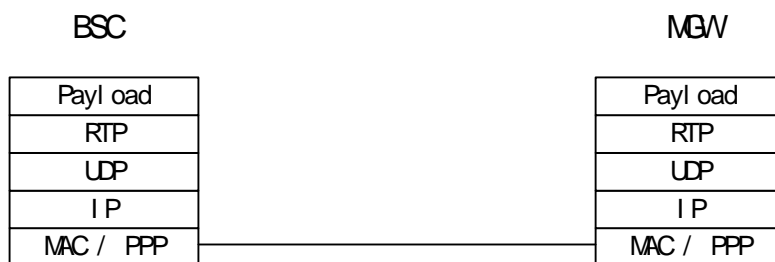
Figure 6.1.1.2.1: User Plane: AoIP protocol stack
