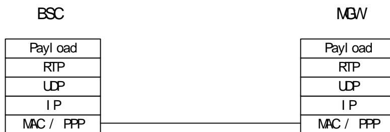
Figure 6.1.1.2.1: User Plane: AoIP protocol stack
