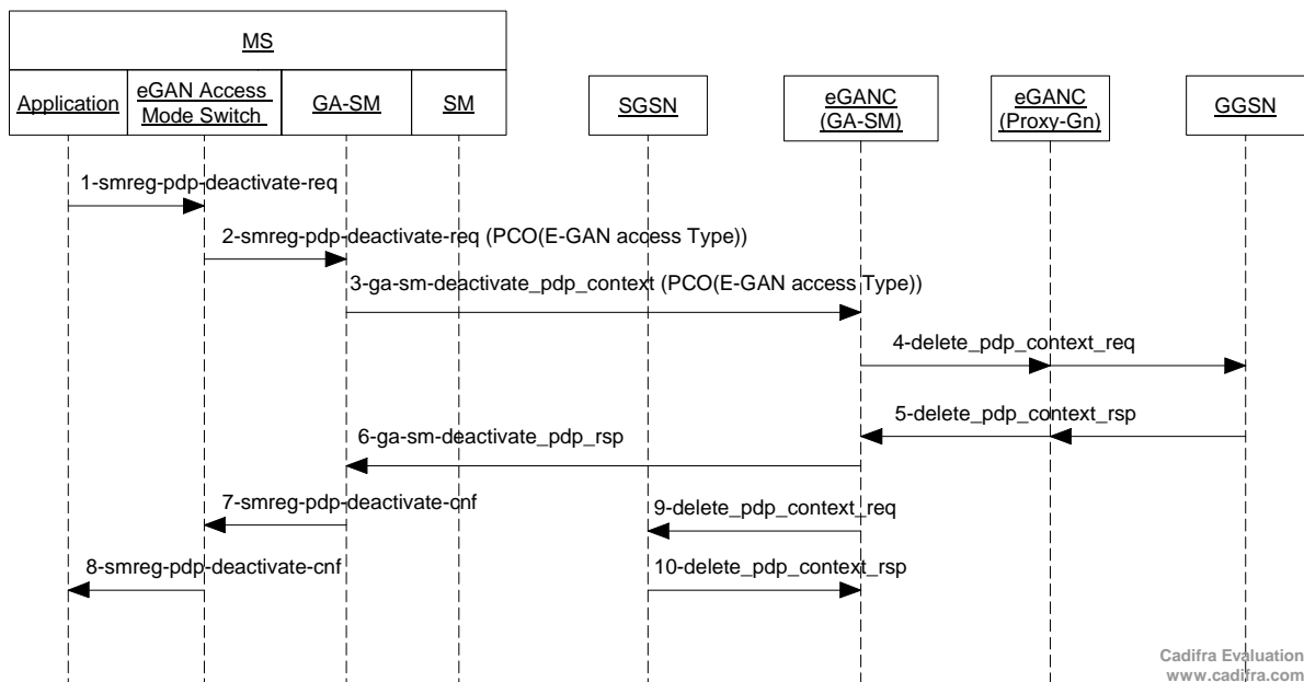
Figure 10: PDP context deactivation procedure on EGAN mode
