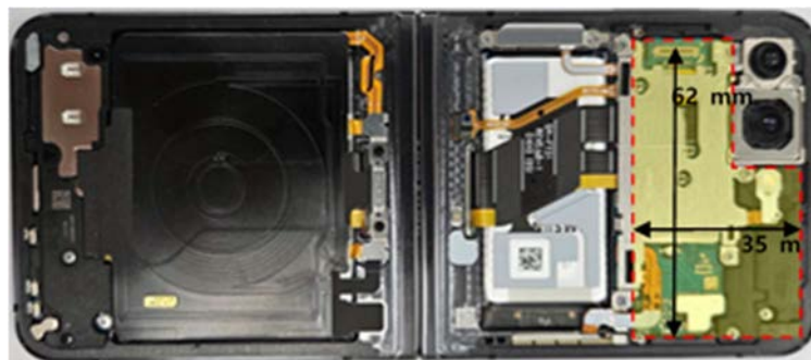
Figure 6.5.2.1-4: Main PCB of a foldable mobile phone.
