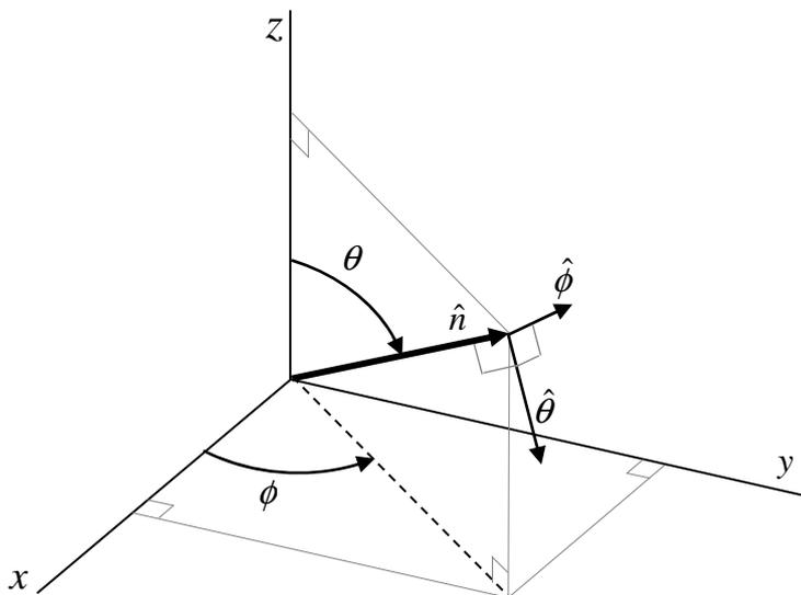
**Figure 7.1.1: Definition of spherical angles and spherical unit vectors in a Cartesian coordinate system, where  $\hat{n}$  is the given direction,  $\hat{\theta}$  and  $\hat{\phi}$  are the spherical basis vectors**
