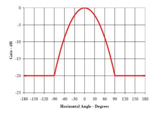
Figure 7.7.4-2 Simplified antenna pattern [ITU-R M.2135].
