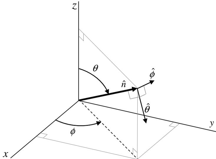
**Figure 7.5-2: Definition of a global coordinate system showing the zenith angle  $\theta$  and the azimuth angle  $\phi$ .  $\theta=0^\circ$  points to zenith and  $\theta=+90^\circ$  points to the horizon. The spherical basis vectors  $\hat{\theta}$  and  $\hat{\phi}$  shown above are defined based on the direction of propagation  $\hat{n}$ .**
