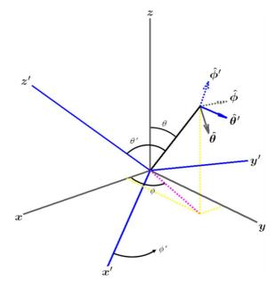
Figure 7.1.3-2: Definition of spherical coordinates and unit vectors in both the GCS and LCS.
