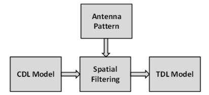
Figure 7.7.4-1 The basic idea for filtering the CDL model to TDL model.
