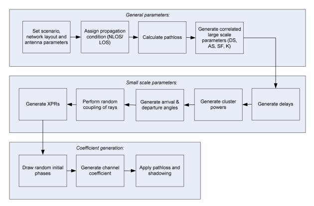
Figure 7.5-1 Channel coefficient generation procedure
