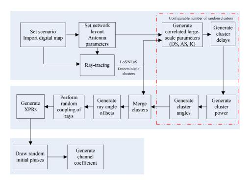
Figure 8.4-1: Channel coefficient generation procedure
