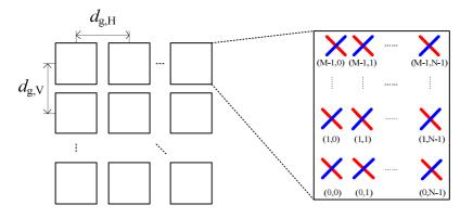
Figure 7.3-1: Cross-polarized panel array antenna model
