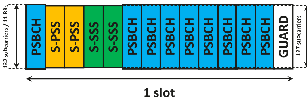
Figure 6.2.2.2-1: Contents of a slot containing S-SSB for normal CP. Each PSBCH symbol contains DMRS.
