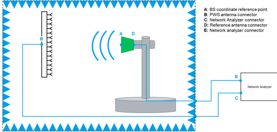
Figure 8.6-1: Path loss calibration in PWS, TX requirements
