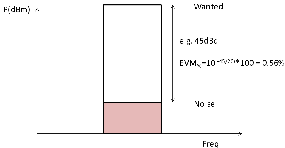
Figure 6.7.1-1: Example of EVM as a power ratio in dB
