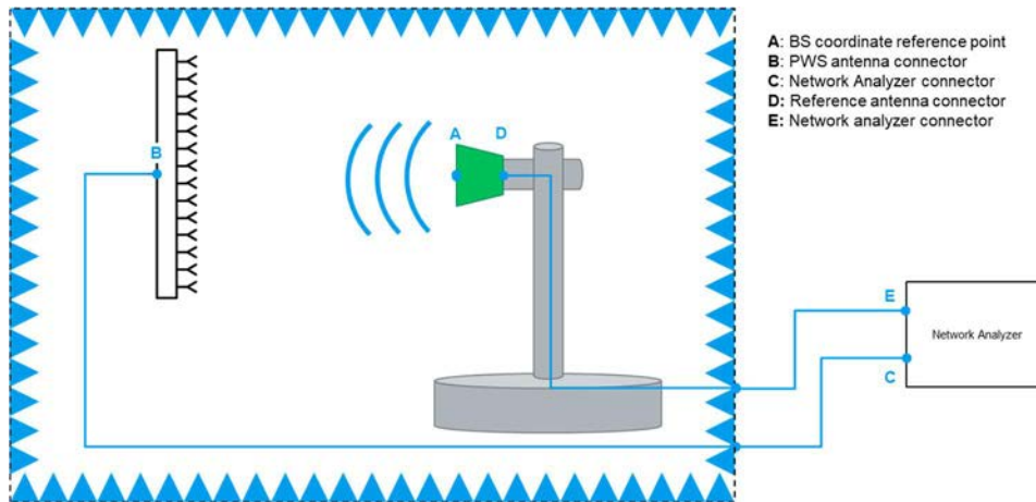
Figure 8.6-1: Path loss calibration in PWS, TX requirements
