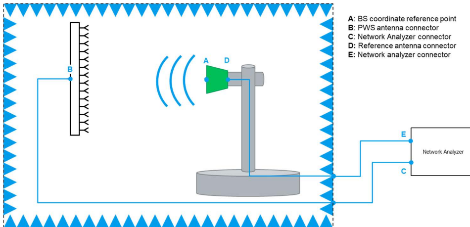
Figure 8.6-1: Path loss calibration in PWS, TX requirements
