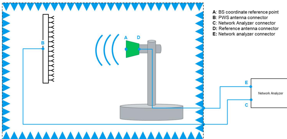
Figure 8.6-1: Path loss calibration in PWS, TX requirements
