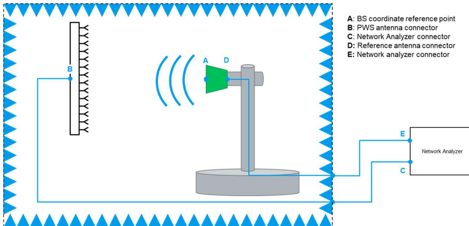
Figure 8.6-1: Path loss calibration in PWS, TX requirements
